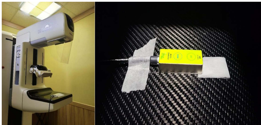
Fig. 2. (Color online) Equipment used for the experiment. Shows the mammography X-ray generator and dosimetry setting. (a) X-ray generator, (b) Solid state detector (Multimeter magicmax RQM).
