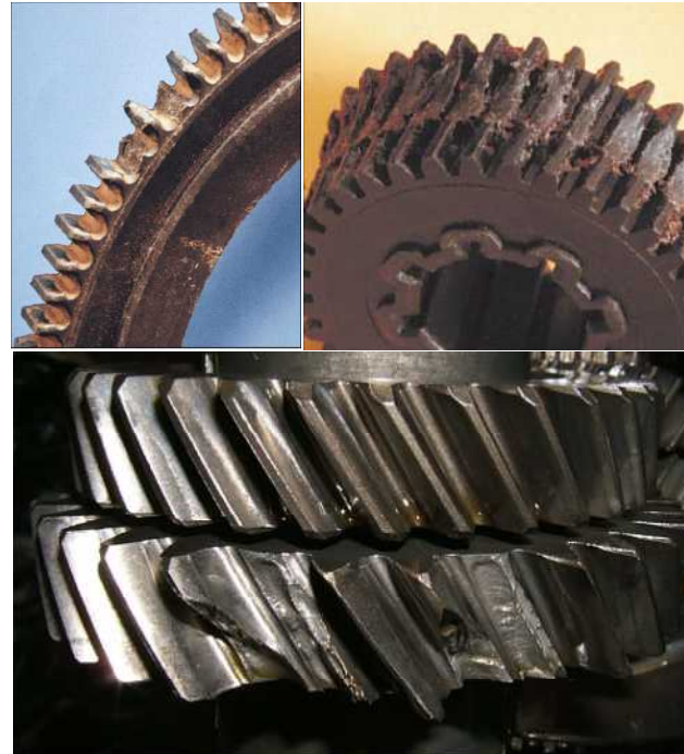
Fig. Broken mechanical gears
